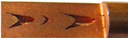
Fig. 9. Chevron crack defects in drawn rod (NORASETHASOPON, 2011). Fig. 10. Cracks on brass CuZn40Pb2 bar contains 0,018 wt. % of antimony (Rajkolhe, 2014).
