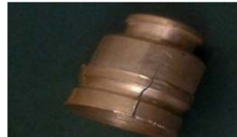
Fig. 12. Jaws marking and cracks in lead brass
