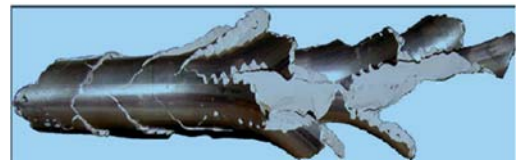
Fig. 9. Chevron crack defects in drawn rod (NORASETHASOPON, 2011). Fig. 10. Cracks on brass CuZn40Pb2 bar contains 0,018 wt. % of antimony (Rajkolhe, 2014).
