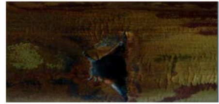
Fig. 3. Porosities and small cracks on brass billet (Mannheim, 2009). Fig. 4. Surface crack on extruded brass bar (PERNIS, 2011).
