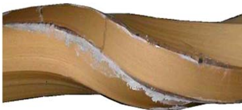
Fig. 5. Distortion of extruded hexagonal bar from brass CuZn40Pb2 (PERNIS, 2011). Fig. 6. Hot tearing in extruded brass rod
