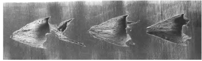
Fig. 7. Extrusion defect (piping) in leaded brass rod (Bauser, 2006). Fig. 8. End cavities in section of leaded brass rod (Bauser, 2006).
