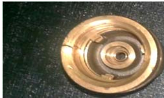
Fig. 11. Hot crack propagation in machined leaded brass
