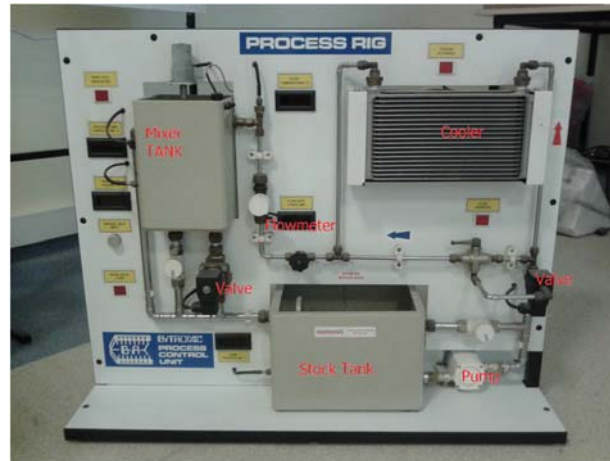
Figure 1: Process Control Training Set
