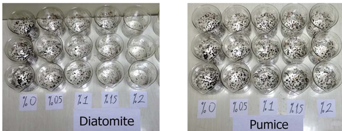
Figure 2. Remaining materials in the glass beakers after the Schellenberg draindown test
