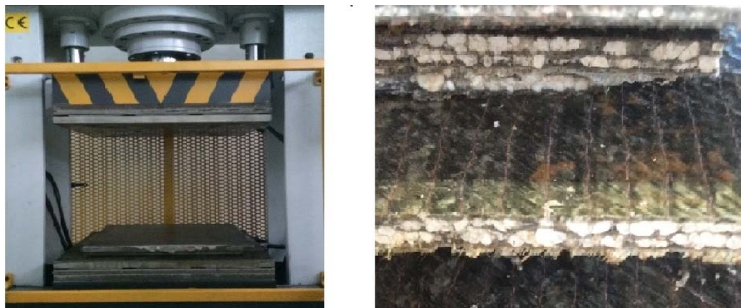
Figure 2. Hot press compression machine and cross sectional view of the composites
