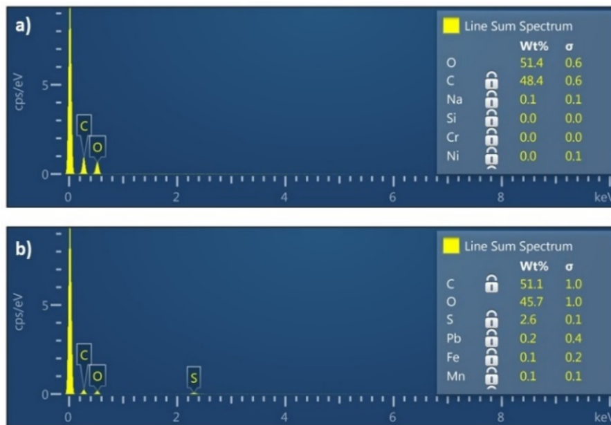
Figure 4. EDS spectra for (a) unmodified cotton and (b) cystamine-modified cotton fibers.
