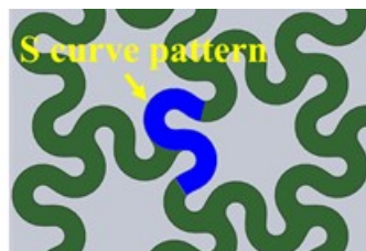
Fig. 3 Example of meshed structure with S curves from basic mesh shape pattern
