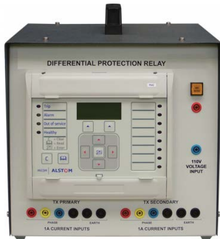
Figure 3. Differential protection relay
